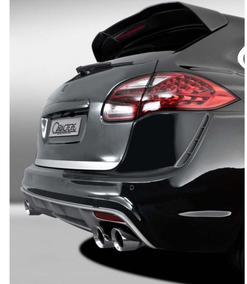
SPORT EXHAUST SYSTEM MADE OF STAINLESS STEEL
