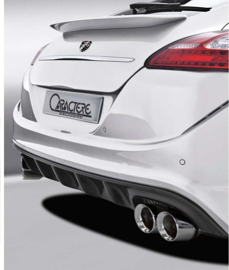
SPORT EXHAUST SYSTEM MADE OF STAINLESS STEEL
